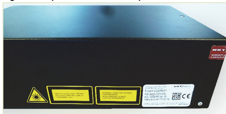
Figure 8 SuperK COMPACT side panel labels
