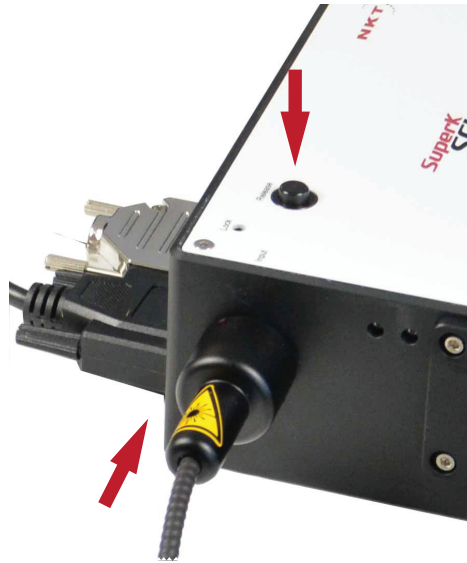
Figure 49 Collimator Installed in a Holder Receptacle
